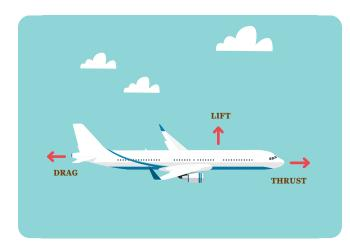
**For something to fly,** lift must be greater than weight, and there must be thrust that can overcome drag.
